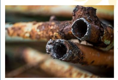
Gradual deterioration of metal due to moisture, air, or chemicals.
